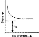
Size Factor: If the size of standard specimen will increase, then the endurance limit of the material will decrease. This is due the fact that a longer specimen will have more defects than a smaller one.
